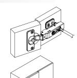
Depth adjustment In 2.25mm
